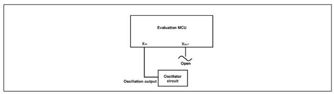
Figure 2.22 External oscillator circuit
